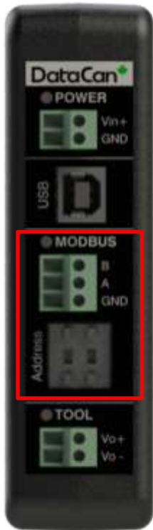
Figure 2: ModBus connection and address selector.
