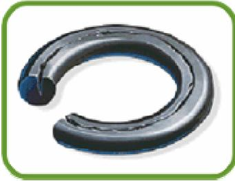
The seal exhibits parallel flat surfaces (corresponding to the contact areas) and may develop circumferential splits within the flattened surface.
