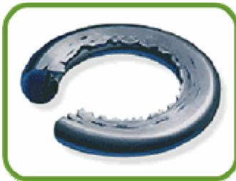
The seal develops ragged edges (generally on the low pressure side) which appear tattered. Excessive seal clearances, excessive pressure, low modulus or hardness elastomers, or improper sizing will lead to an extruded seal.
