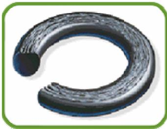
The seal or parts of the seal exhibit a flat surface parallel to the direction or motion. Loose particles and scrapes may be found on the seal surface. Rough sealing surfaces, excessive temperatures, environments containing abrasive particles, or poor elastomer surface finish may lead to an abrasion failure.
