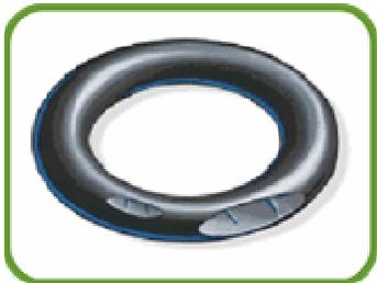
The seal or parts of the seal may exhibit small cuts, nicks or gashes. Sharp edges on the glands or components, improper sizing, or a low modulus/hardness elastomer may lead to installation damage.
