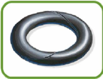
The seal exhibits cuts or marks which spiral around its circumference. Difficult or tight installation clearances with out proper lubrication may lead to this mode of failure. Excessive gland width is also a known cause.
