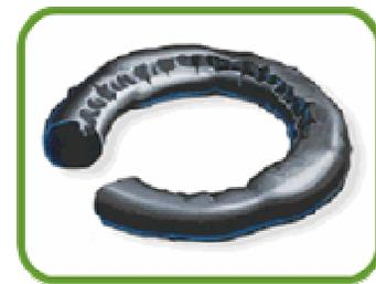
The seal may exhibit many signs of degradation including blisters, cracks, voids or discoloration. In some cases, the degradation is observable only by measurement of physical properties.
