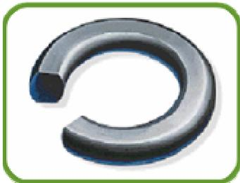
The seal exhibits a flat-sided cross-section, the flat sides correspond to the mating seal surfaces. Excessive compression and temperature, excessive volume swell in chemical, and specific elastomers with high compression set lead to this failure mode.
