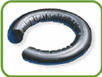
The seal may exhibit radial cracks located on the highest temperature surfaces. In addition, certain elastomers may exhibit softening, or a shiny surface as a result of excessive temperatures.
