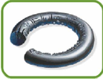
The seal exhibits blisters, pits, or pockets on its surface. Absorption of gas at high pressure and the subsequent rapid decrease in pressure results in gas that was once trapped inside the elastomer to explosively decompress and exit the seal. The absorbed gas blisters and ruptures the surface as the pressure is rapidly removed.
